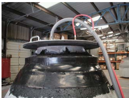
Riser-Wrap® Vacuum Test
